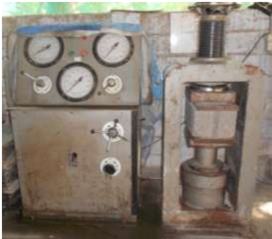
Figure 8: Compression Testing Machine with arrangement of laying block
