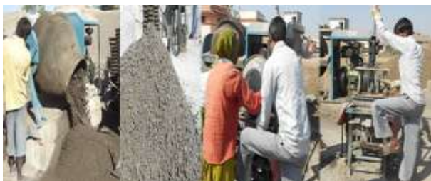
Figure 5: Lean concrete produced and casting machine (mould-vibrator assembly)
