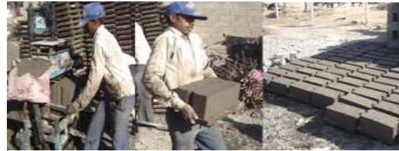
Figure 6: Concrete pressed in the machinery and are stacked for sun-drying
