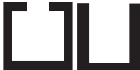
Figure 1 Two possible shapes of open-loop resonator.
