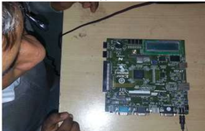
Fig 4: - (a) Block diagram of system, (b,c) FPGA Board with microphone. This system is based on audio input of sparten-3 based FPGA board which is digitized and interfaced with sparten-3 FPGA processor. This processor is used to process the digitized audio input and extract the voice activity signal. This signal is processed to generate the MFCC coefficient which is pass through HMM filter for getting the feature database and
