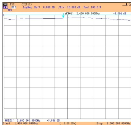
Fig 7. Measurement result of insertion loss ( S_{12} )
