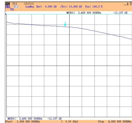
Fig 8. Measurement result of isolation ( S_{32} )
