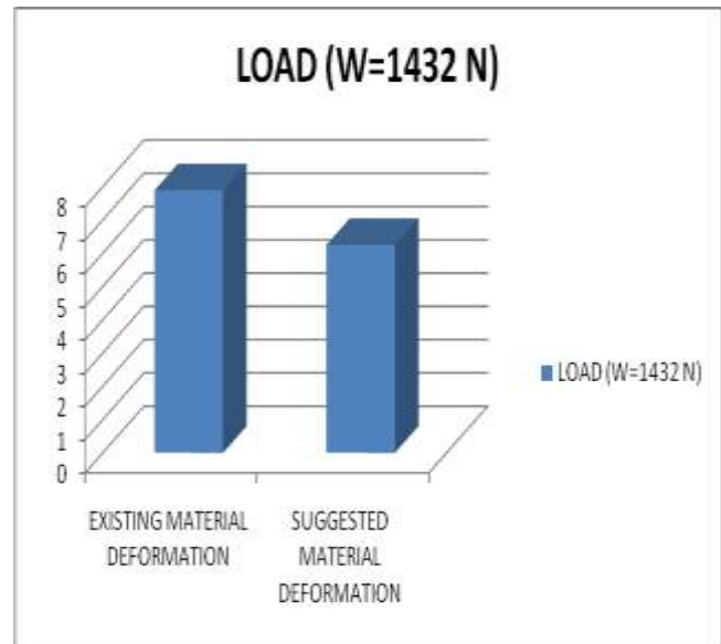
Fig 5.1. Reduction in deflection for load of single person
