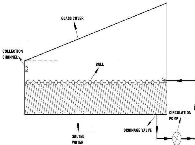
Fig.5: Schematics of the extended surfaces solar still.
