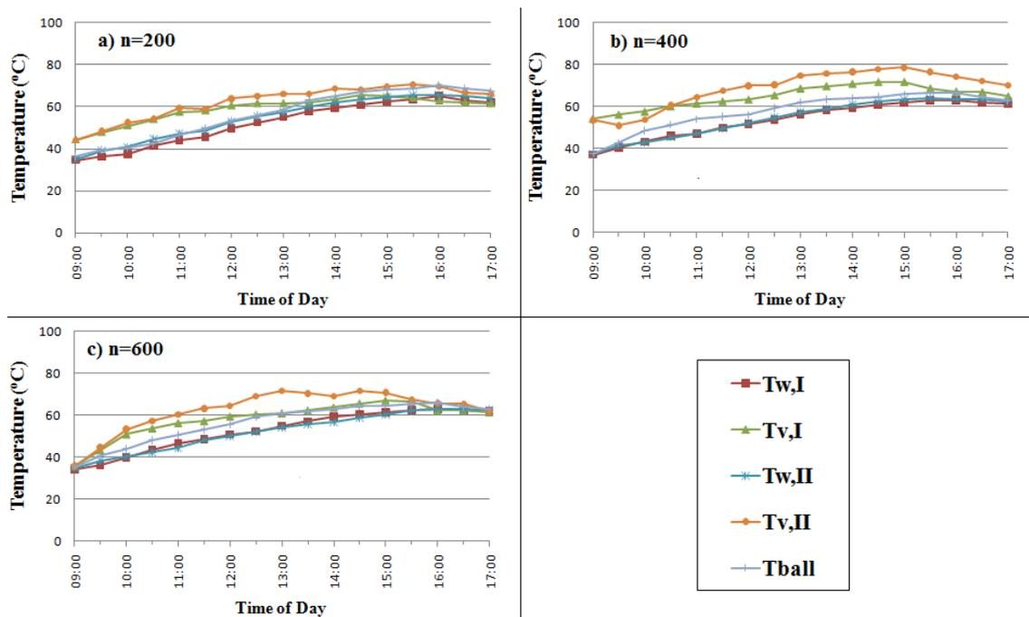
Fig.10: Variations of temperatures of water and steam temperature (for the moving balls)
