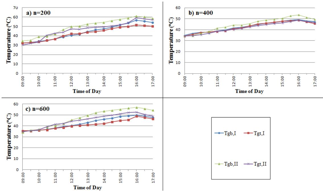
Fig.7: Variations of the temperatures of the condenser glass (for the stationary balls)
