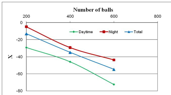
Fig.15: Comparison of productivity rate between conventional system and distiller with stationary balls
