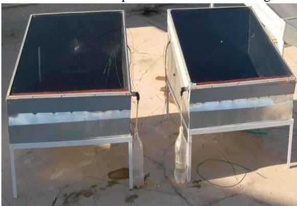
**Fig.1:** Photograph of the experimental solar stills
