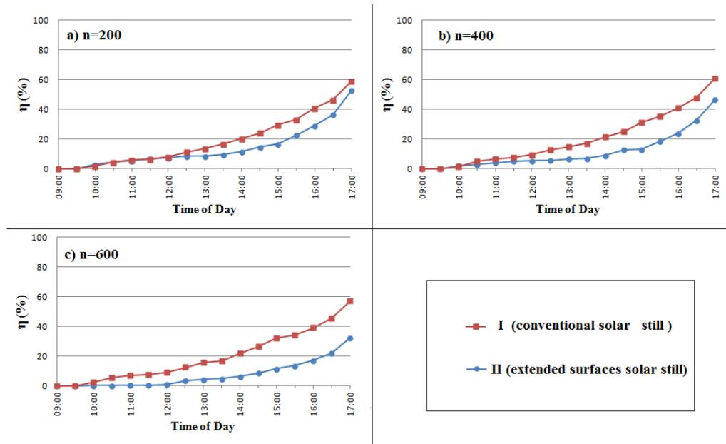
**Fig.13:** Variations of the efficiency of solar still (for the stationary balls)
