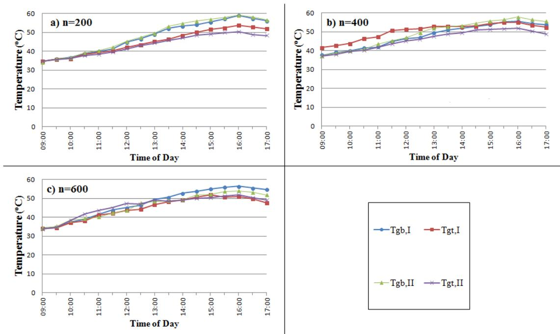
Fig.8: Variations of the temperatures of the condenser glass (for the moving balls)
