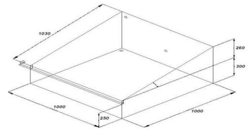
**Fig.2:** Schematics of the solar still.
