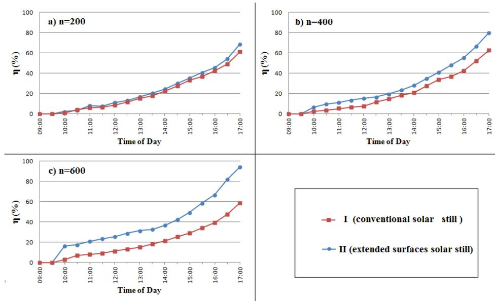
**Fig.14:** Variations of the efficiency of solar still (for the moving balls)
