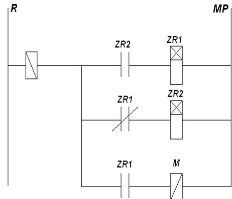
**Fig.4:** Schematics of Control circuit
