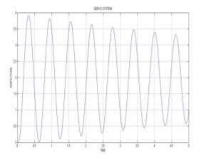
Overshoot of the system can be reduced by 78.19%, when corrected by critical oscillation, and 94.20% when corrected by 11:4 convergent oscillation. However lifetime is hardly affected, no matter which correction is used.
