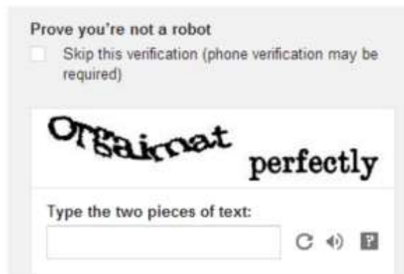
Figure 1 text-based CAPTCHA used by Gmail account creation process. A user must enter each displayed character correctly in-order to proceed. The volume icon indicates that a user may elect for an audio-based CAPTCHA test.[2]
