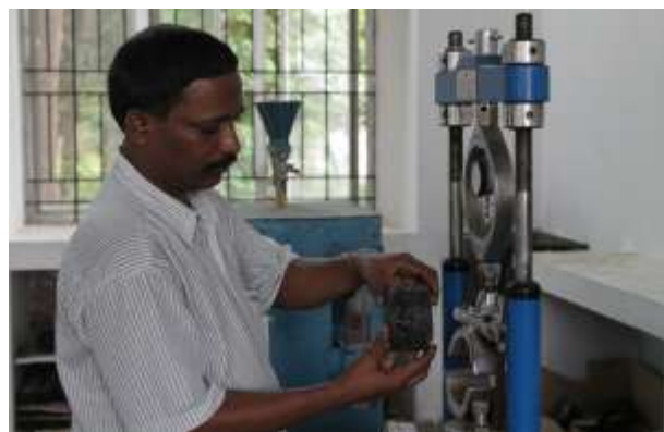
Fig. 3.1 Testing of casted mould with Marshall Stability Testing Machine
