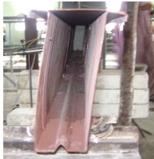
Figure 16 Torsional buckling of STHAT155B
