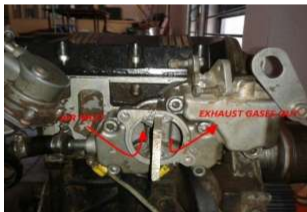
Figure 1.4: Modified Inlet and Exhaust Manifold of Six Stroke Engine
