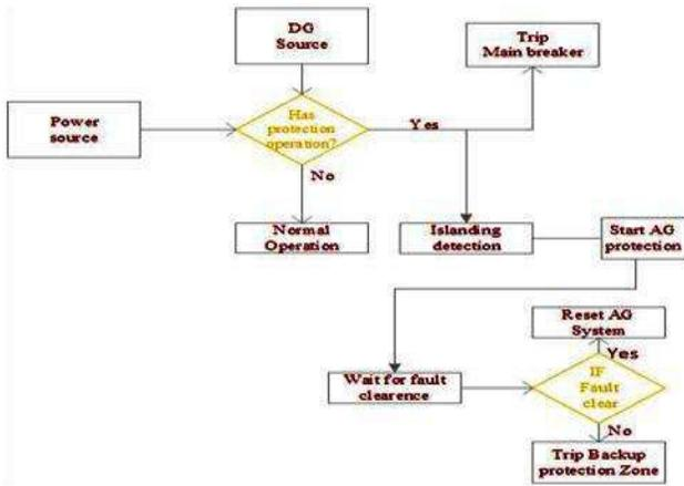
Fig.4. Flow chart of the anti-islanding protection
