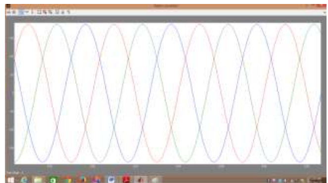
Fig.15. Three phase stator voltages
