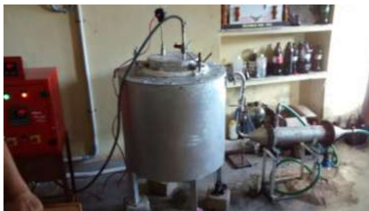
Fig. 2 photo graphic view of fast pyrolysis plant
