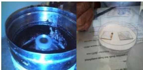
b) Images showing spin coating deposition of prepared ODCB suspension deposited glass substrates
