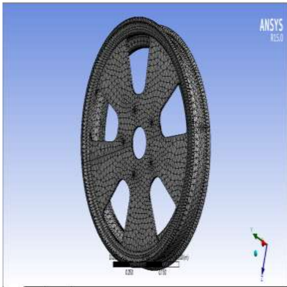
Figure 4 Meshing of Wheel Rim
