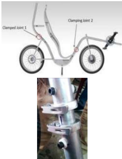
Fig. 1. Frame of HPV and clamp design
