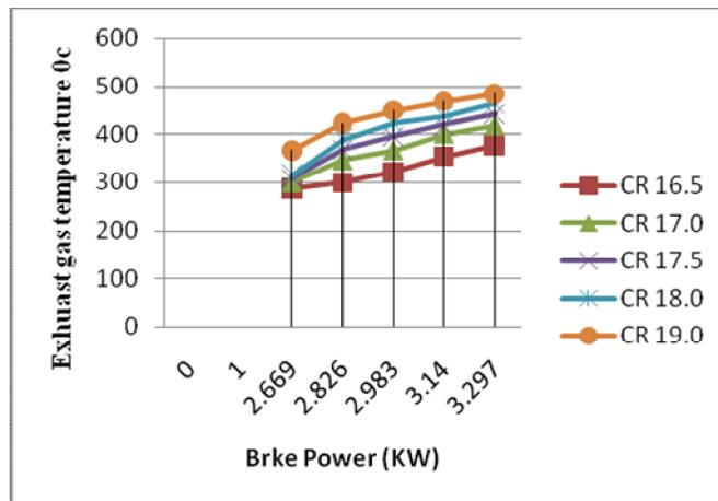
Exhaust gas temperatures were found to be increasing with the increase in load and the compression ratio. The highest exhaust gas temperature was recorded for the compression ratio 19.0 while the least was for 16.5.
