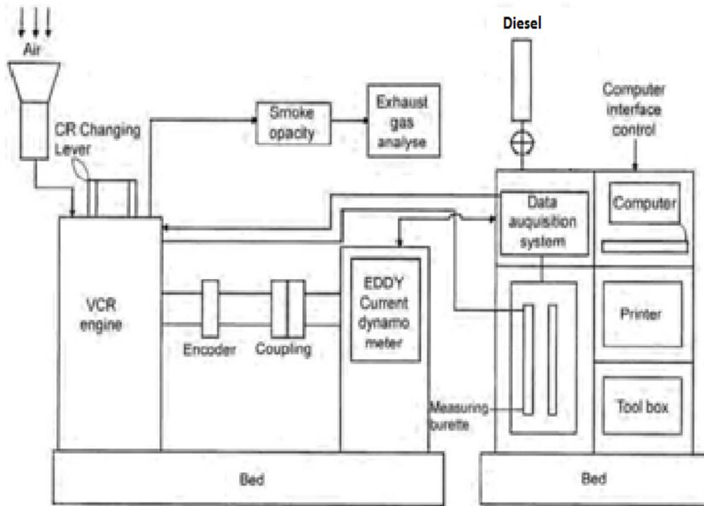
Figure 3.1: Block Diagram of VCR Engine
