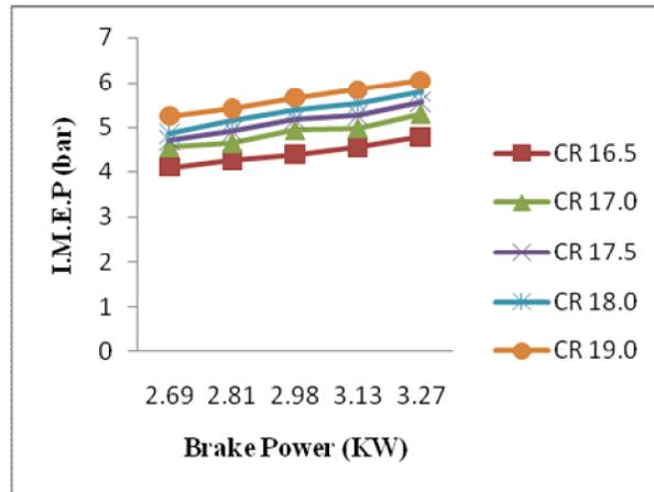
Indicative Mean Effective Pressures were found to be increasing with the increase in load and the compression ratio. The highest Indicative Mean Effective Pressures was recorded for the compression ratio 19.0 while the least was for 16.5.
