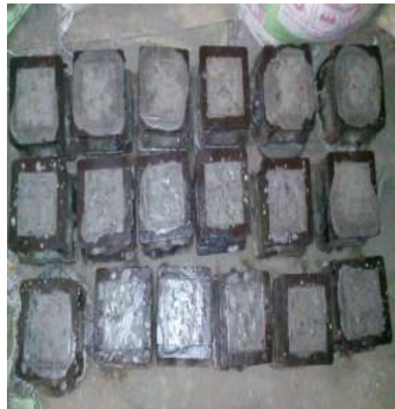
Figure.2 casting of specimens
