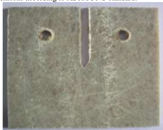
Fig. 1 Hybrid composite of 50% glass and 50% jute fibre
