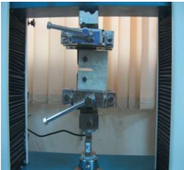
Fig. 2 Compact tension specimen fitted the UTM
