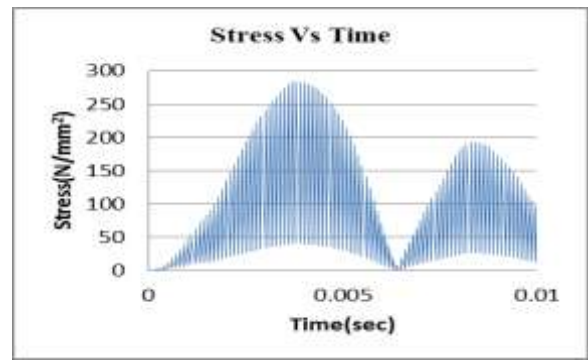
Fig 8: Stress Vs time for metallic sandwich
