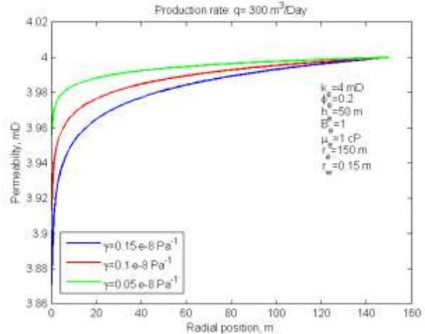
Fig. 7 Effect of permeability modulus on permeability
