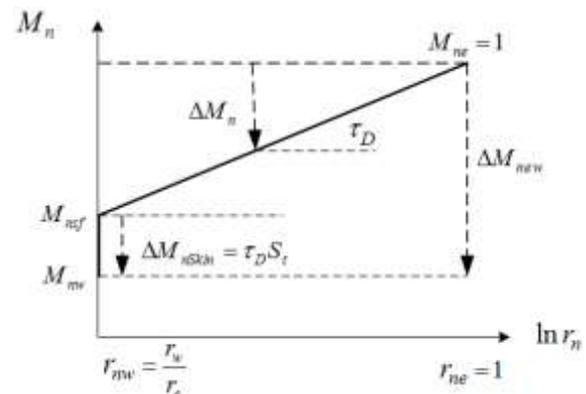
Fig. 1 Mobility function ( $M_n$ ) vs. radial distance for production
