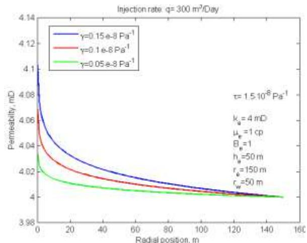
Fig. 8 Effect of permeability modulus on permeability
