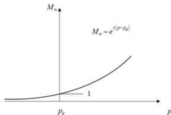
Fig. 4 Mobility function vs. pressure
