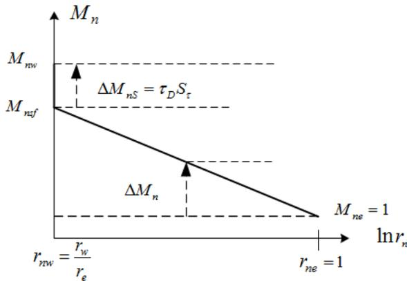
Fig. 2 Mobility function ( $M_n$ ) vs. radial distance for injection
