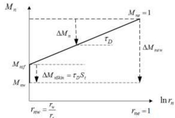
Hence, one may define an apparent wellbore radius,  $r_{aw} = r_w e^{-S_\tau}$ . The apparent wellbore radius may be thought of as a fictitious radius which makes the wellbore mobility without skin equal to the wellbore mobility with skin. The concept is illustrated in Fig. 3.
