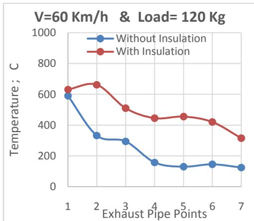
Fig. (12) Temperature distribution at 60 Km/h car speed and load of 120 Kg.
