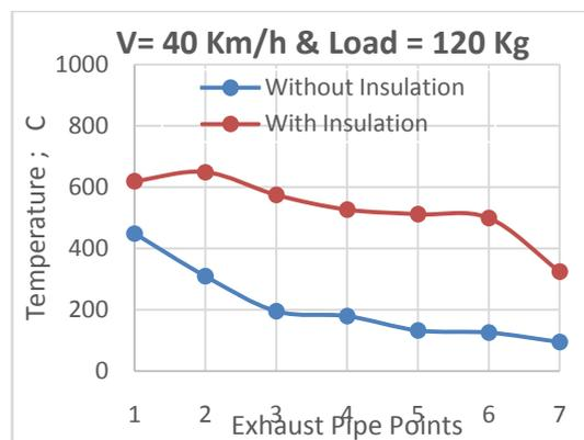
Fig. (10) Temperature distribution at 40 Km/h car speed and load of 120 Kg.
