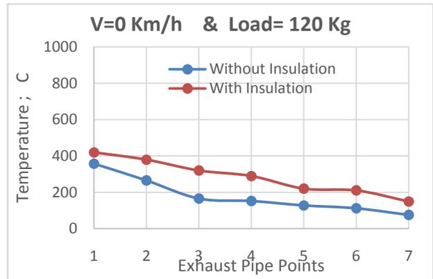
Fig. (8) Temperature distribution at zero car speed and load of 120 Kg.
