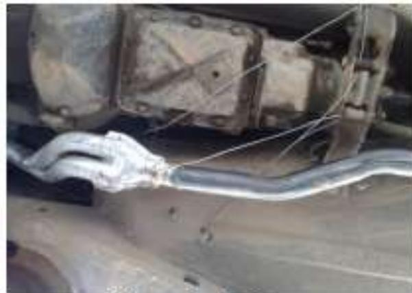
Fig. (5) Exhaust pipe without insulation.
