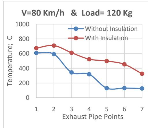
Fig. (14) Temperature distribution at 80 Km/h car speed and load of 120 Kg.
