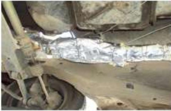
Fig. (6) Exhaust pipe with Insulation.
