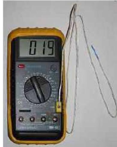
Fig. (4) Thermocouple with display unit.
