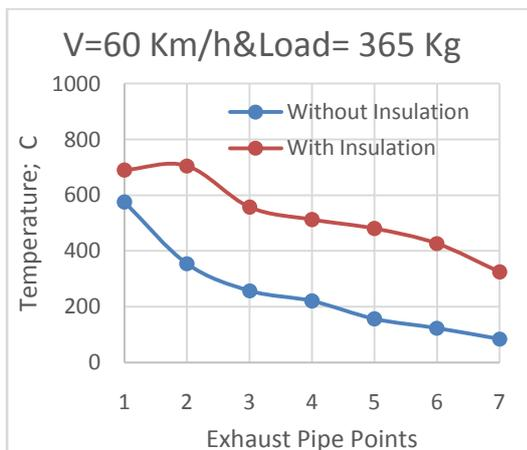
Fig. (13) Temperature distribution at 60 Km/h car speed and load of 365 Kg.
