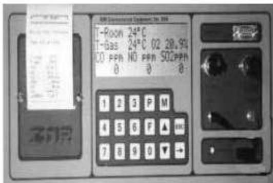
Fig. (7) Photograph of IMR® 2800 Backlit LCD & Keypad [14].
