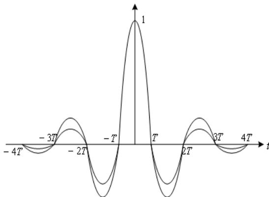
Figure 6- Impulse response of RC filter
