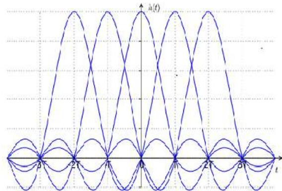
Fig 4- Raised cosine impulse showing zero ISI property [7]
