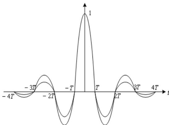
Figure 6- Impulse response of RC filter
