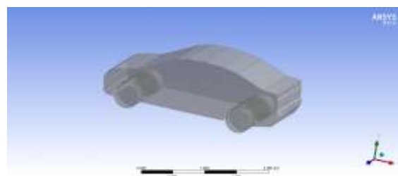
Fig.5.1. SUV geometry model without spoiler
