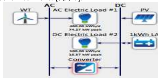
Fig. 4. Standalone ac/dc-bus type HPS
