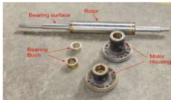
Fig 2. The bearing system for an 6” water cooled Submersible motor (Courtesy: VIRA PUMPS, Kolhapur INDIA)
