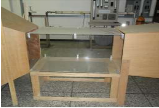
Fig. 2 Transparent test section chamber
