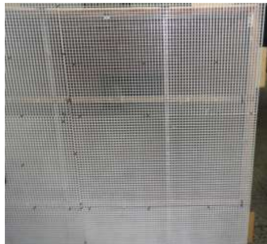
Fig. 5 The settling chamber.
