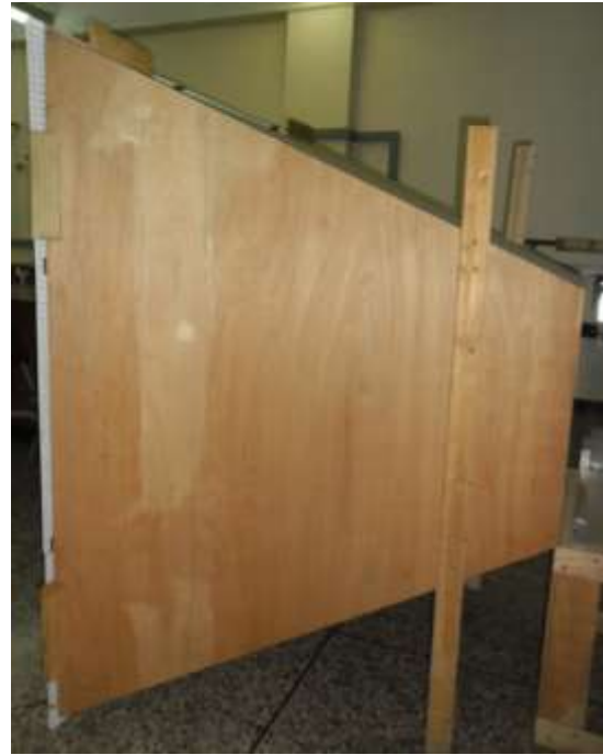
Fig. 4 The contraction cone assembly.
