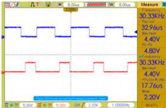
Fig. 19. Output voltage during buck operation.
