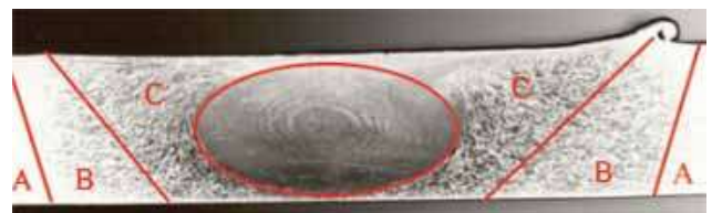
Fig.3 Microstructural zone classification in a friction stir welding.
