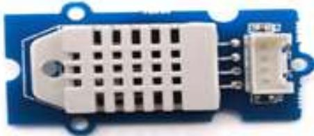
Fig. 8 Temperature and Humidity Sensor
