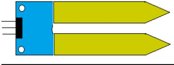
Fig. 7 Soil Moisture Sensor
