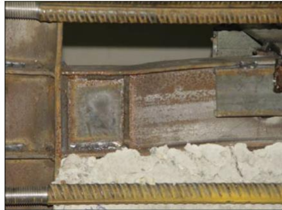
(b) Plastic hinge in the top beam.
