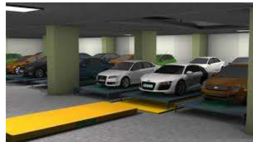
Fig. 3 Cart Type Parking System
