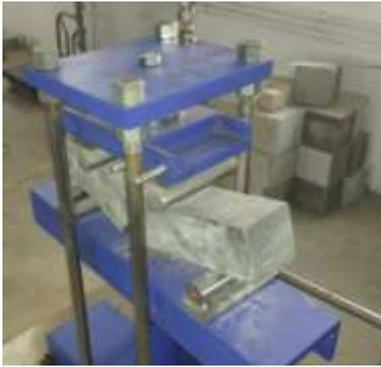
**Fig-6:** Flextural Test.
