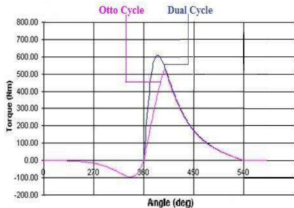
Fig.7 Torque-crank angle diagram for four stroke engine
