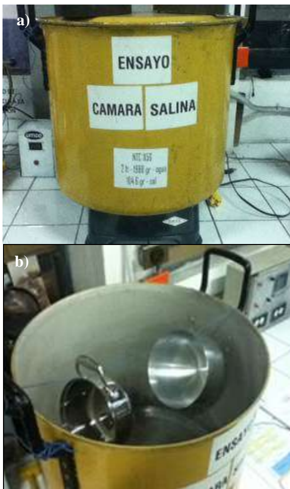
Fig. 1. a) Image of the salt spray chamber for material corrosion test. b) Image of two pots suspended in the salt spray chamber.
