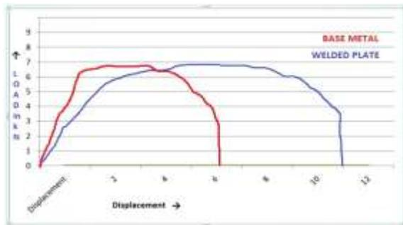
**Figure 15 Tensile Test for Base Metal & Welded plate**
