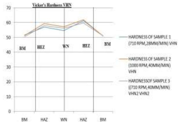
Figure 13 Micro Hardness for Samples
