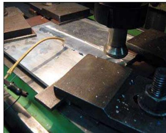
Figure 4 Friction Stir Welding Process
