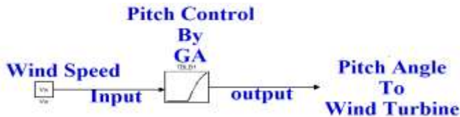
Fig. 9 Pitch angle \beta Vs wind speed V_w as a block in Mat lab/Simulink..
