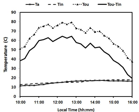
Figure 6: Variation of ambient, inlet, outlet temperatures and wind speed with time
