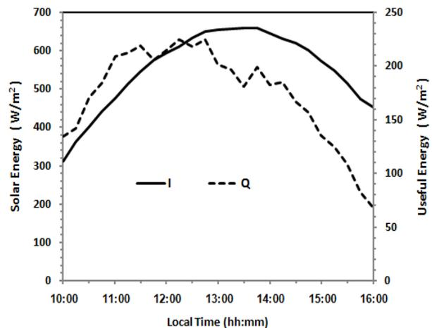
Figure 4: Variation of the Solar Radiation ( $I$ ) and the useful heat gained ( $Q_u$ ) with time
