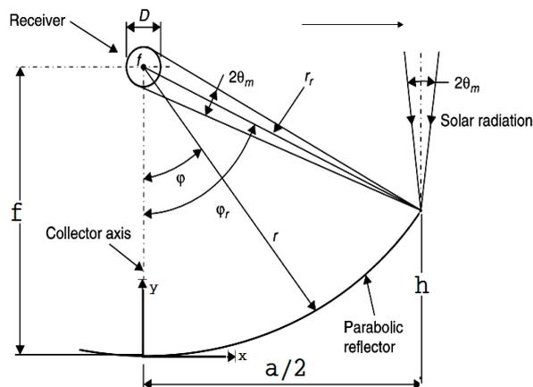
Figure 1: Cross-section of the PTC with circular Receiver
