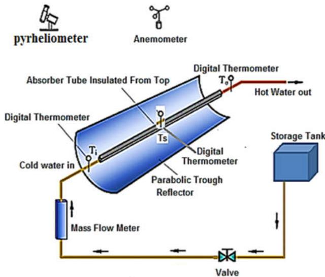
Figure 3: Schematic diagram of the experimental work
