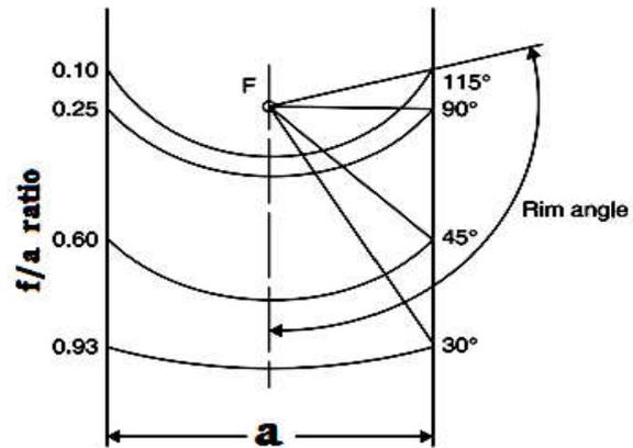
Figure 2 : parabola focal length and curvature
