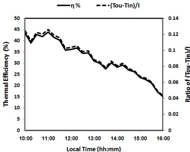
Figure 5: Variation of the Thermal efficiency ( $\eta$ ) and the ratio of  $(T_{ou} - T_{in})/I$  with time
