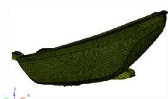
Figure 5. Headlamp meshed model using Hyper mesh
