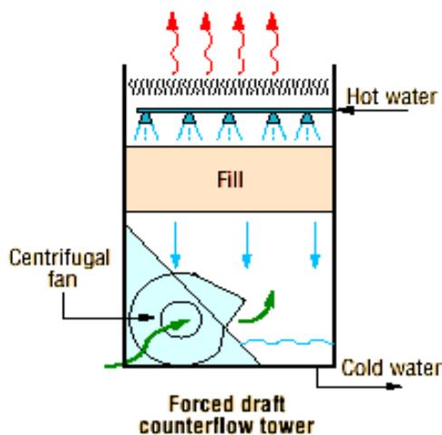
Fig. 2.5 Counter flow forced draft
