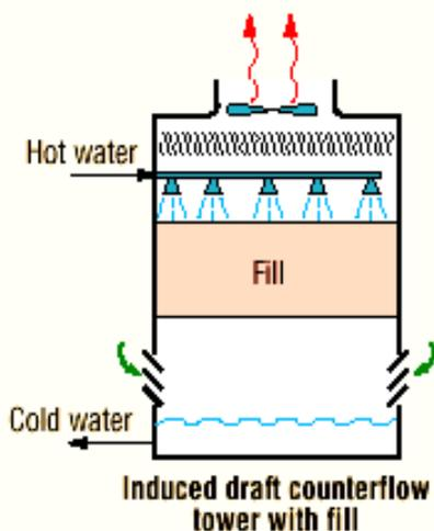
Fig. 2.6 Counter flow induced draft
