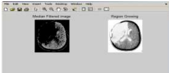
Figure 4.4 Filtering and Region Growing Image The figure 4.4 shows filtering and region growing Image. The region growing is the process of growing of region based on intensity values. Initially the pixel was chosen and growing of pixel takes places with the help of their intensity values.
