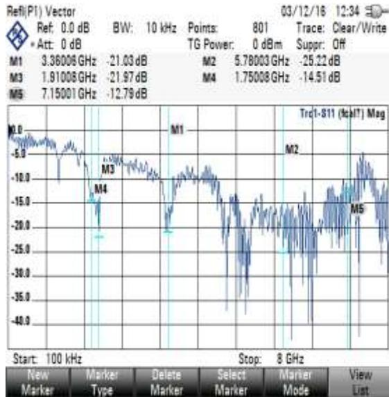
Fig 11. Measured result of sub patch 2 with loading 21
