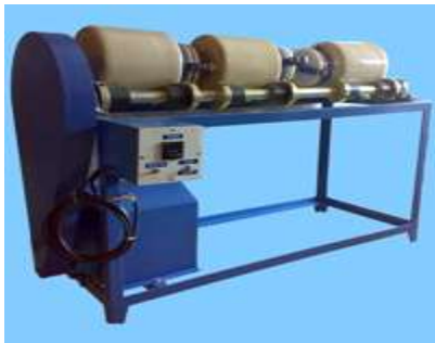
Fig. 2 Ball and Jar mill.
