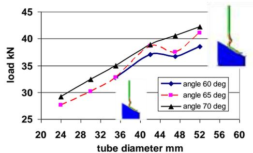
Fig.5 Tube diameter vs forming load for three different half die angles
