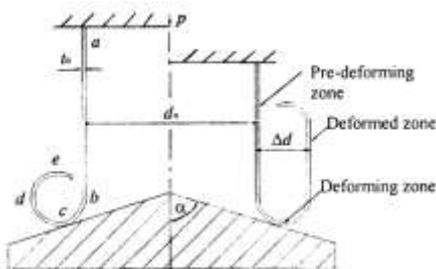
Fig. 1 A sketch of tube inversion process by conical die
