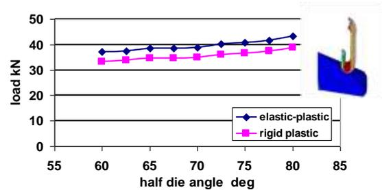
Fig.4 Half die angle vs forming load
