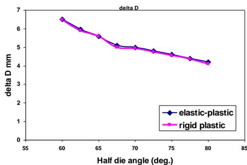
Fig. 3 Double-walled tube gap Δd vs the half die angle
