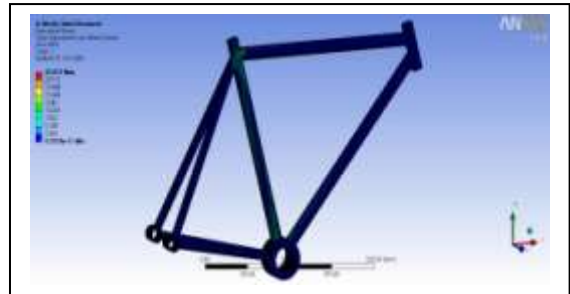
Figure 25:- Equivalent stress, Vertical impact
