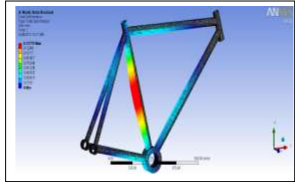
Figure 41:- Horizontal impact (maximum deformation), Aluminum 7005-T
