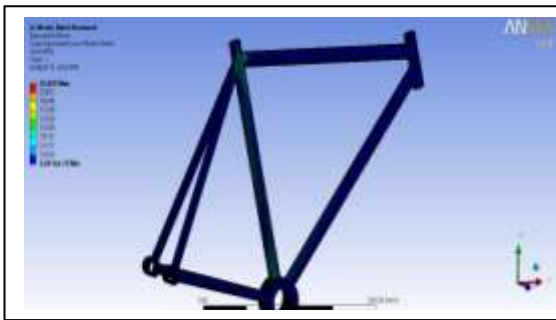
Figure 35:- Equivalent stress, Vertical impact
