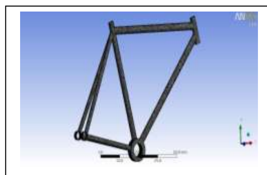
Figure 2:- Bike frame with meshing of 5mm
