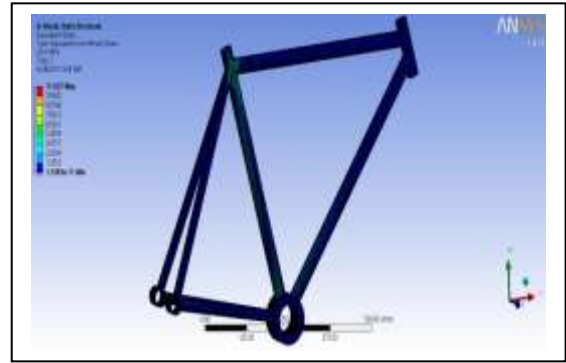
Figure 24:- Equivalent stress, Steady state pedaling
