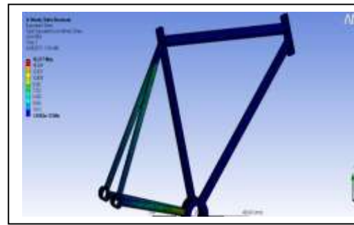
Figure 32:- Equivalent stress, Rear wheel braking
