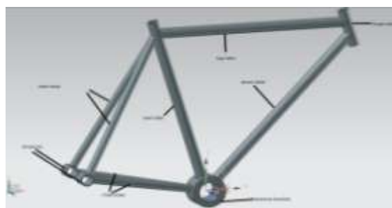
Figure 1:- Tubing diagram of the bike frame
