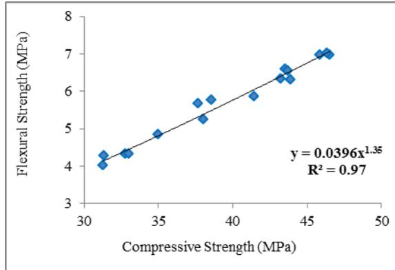
**Fig Error! No text of specified style in document.: Relationship between Compressive Strength and Flexural Strength of Polyester Fibre Reinforced Concrete**
