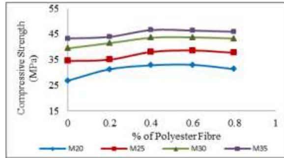
Fig 1: Compressive Strength Vs Percentage of Polyester Fiber Reinforced Concrete
