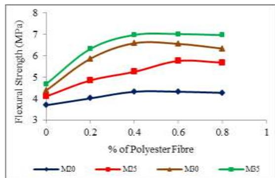
Fig 2: Flexural Strength Vs Percentage of Polyester Fiber Reinforced Concrete
