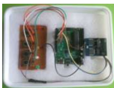
Fig. 4. Basic connections of Arduino Uno and EMIC2
