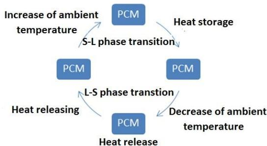
Phase change materials are substances characterized by ability to phase transition at certain temperature range. Scheme of the phase change transition is presented on figure 1. During phase transition there is always heat emission or heat absorption which is called latent heat of fusion. Temperature of transition and amount of latent heat of fusion are distinctive for each material.
