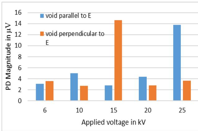
Fig.5: Comparison of PD magnitudes with different applied voltage for the model shown in Fig 1 and Fig 2.
