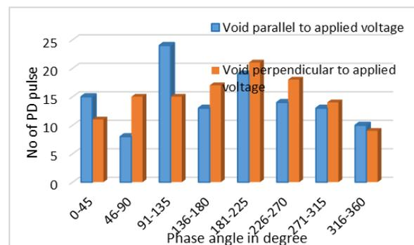
Fig 8: Number of PD pulse for different phase angles
