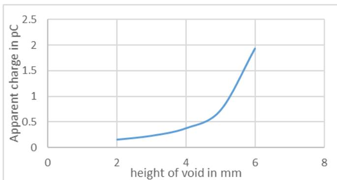
Fig. 6: Variation of apparent charge with height of the void
