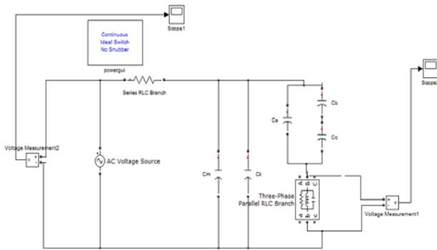
**Fig 1:** Model of a cylindrical void within a solid insulation shows its axis parallel to the applied electric field
