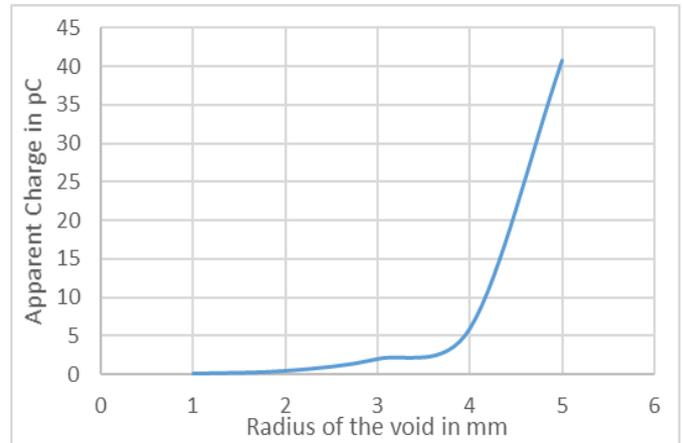
Fig. 7: Variation of apparent charge with radius of the void
